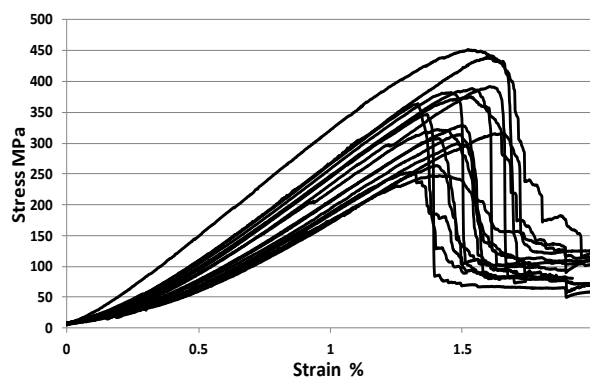
Figure 4. Scattering of GFPP yarns tensile behavior (200mm gauge length, 1.67 \cdot 10^{-4} \text{ s}^{-1} strain rate)
