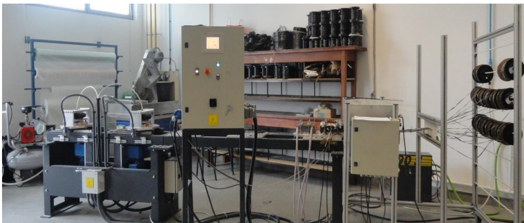
Figure 4. Developed prototype pultrusion line
