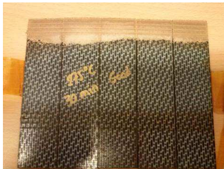
Figure 2. Triangular energy directors moulded on the surface of the adherends. The darker colour of the PPS resin in the energy directors evidences some oxidation.
