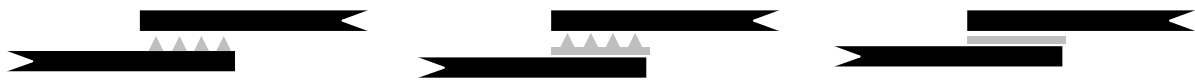
Figure 1. Types of energy directors used in this study. Left: four triangular ridges moulded on substrate (4TM); middle: four triangular ridges moulded on a loose resin stripe (4T); right: flat energy director
