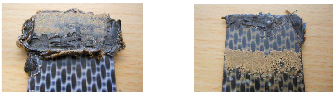
Figure 11. Mating fracture surfaces for a 4TM welded sample (500 N, 86.2 \mu m, 0.75mm)
