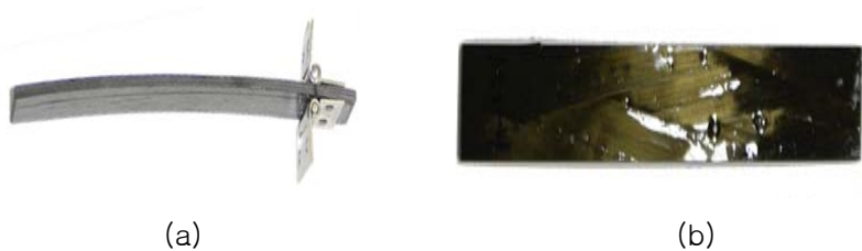
Figure 3. Shape of specimens (a) Mode I (b) Mode II
