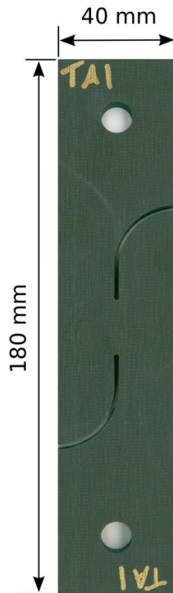
Figure 1. Pin-loaded tensile specimen used for experimental investigation.
