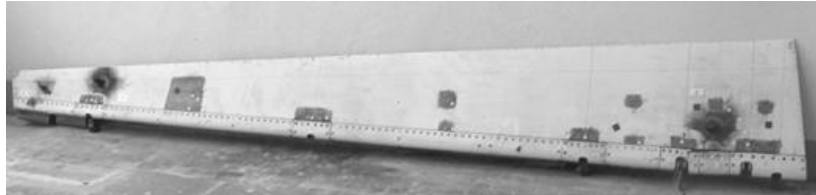
Figure 1. Elevator after the impact of a lightning bolt at the end of the static test.
