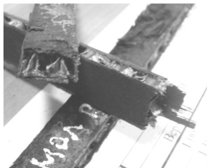
Figure 12. The character of destruction of a sample below the impact zone
