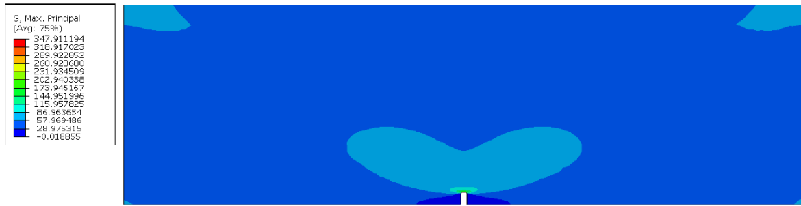
Figure 6. Stress distribution on the notched laminate computed through the present multiscale approach.
