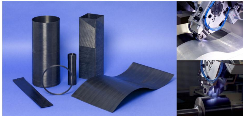
Figure 1. Process and shape diversity of laser-assisted tape placement
