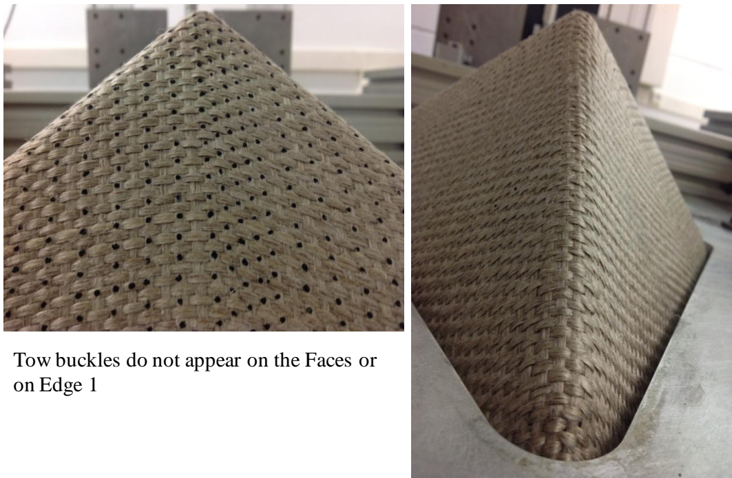
Figure 5: Plain weave fabric: Face C and Edge 1 using the specially designed blank holder set
