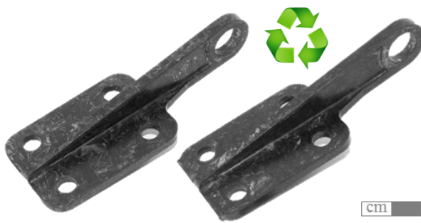
Figure 5. Original door hinge (left) versus recycled door hinge (right).
