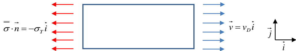
Figure 3. Tensile test in a translating frame
