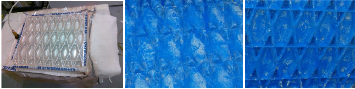
Figure 5. Aluminum male mold and vacuum bag (left) for preparation of double-carpet rubber tool: volumetric part (center) and geometric part (right).
