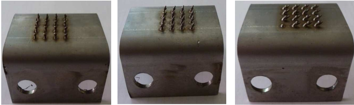
Figure 7 Pin arrays after failure of the KS-2 joints under normal (left), mixed (center) and shear (right) load
