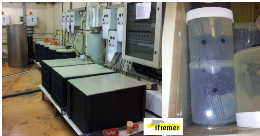
Figure 3. Ifremer facilities, sea water ageing baths with natural water pumped from the sea.
