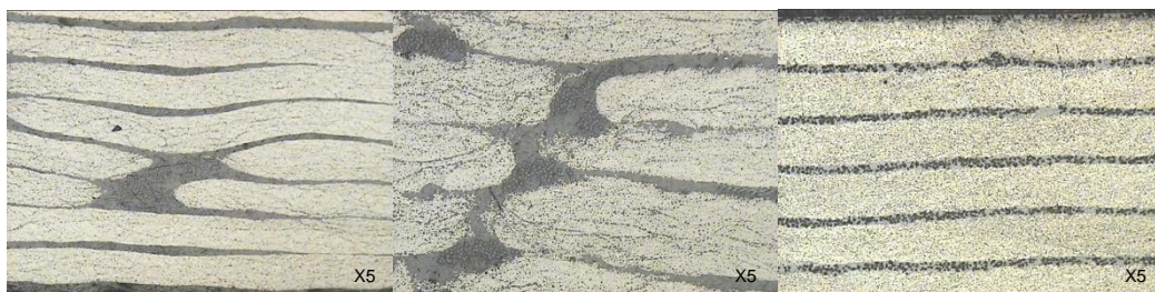
Figure 2. Optical microscope observation on UD samples Infused, RTM and Pre-preg material (left to right)
