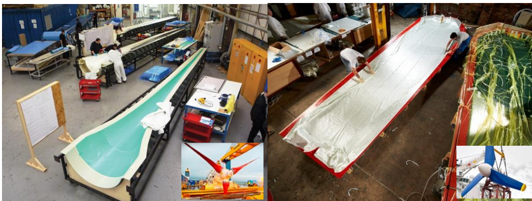
Figure 1. On left, the Gurit tidal turbine blade for the HS1000, on right the Atlantis blades manufactured by Norco, sources: Gurit and Norco
