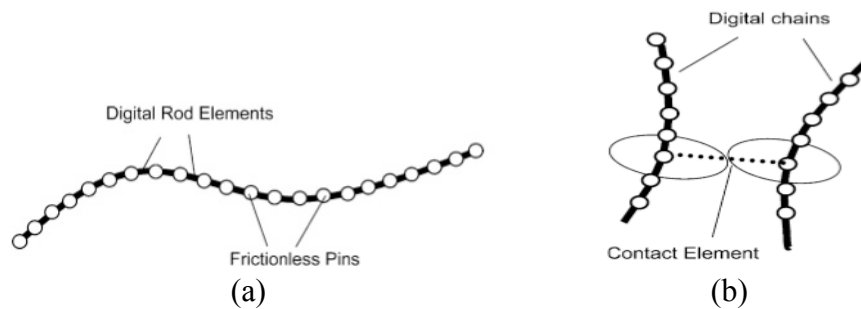
Figure 1: Schematic of a single digital chain (a) and two digital chains (b) interacting through a contact element.
