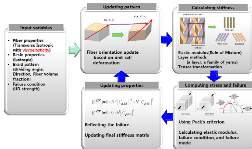
**Figure 1.** Schematic diagram describing new numerical method to calculate the stress based on strain increment.
