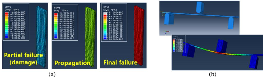
**Figure 2.** Numerical analysis model. Tensile test model (a) and bending test model (b). SDV1 is partial failure variable and SDV2 is final failure variable.
