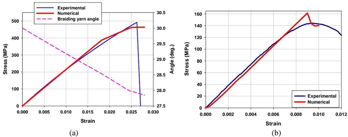
Figure 3. Comparisons between numerical and experimental results. (a) tensile and (b) bending tests.
