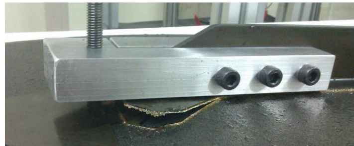
Figure 4: Picture of stringer debonding process
