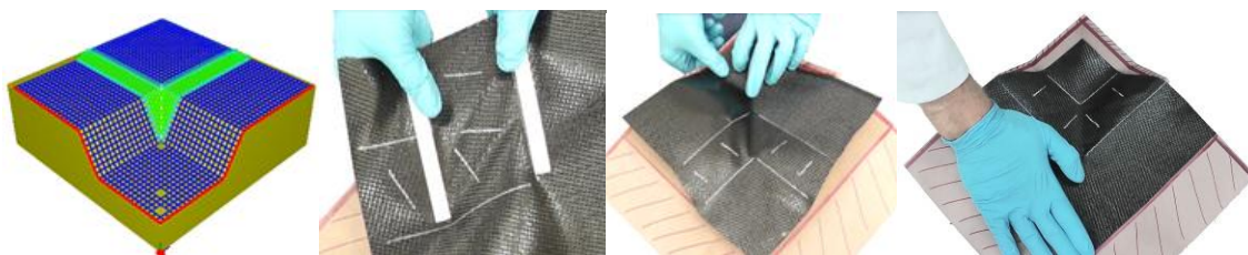
Figure 4: (Left to right): The VFP deformation diagram. Preshearing the material using ‘edge clamping’. showing the marked shear area. Presheared ply being applied to task A and already fitting into the tool recess. Presheared ply being applied to task B and already fitting into the tool recess
