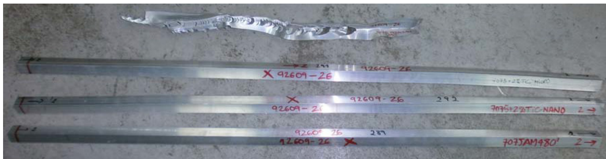
Figure 4. L aluminium profiles extruded in pilot plant
