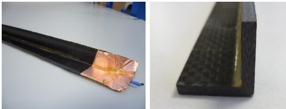
Figure 6. Showing an image of the electrically L-shaped stiffener, detailing the contact arrangement, and showing the consolidation and degree of resin bleed via the image of a cut end.
