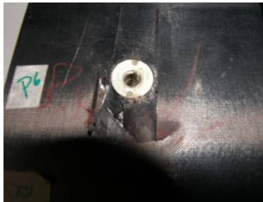
Figure 6. Top-view of failed specimen of P6 insert.
