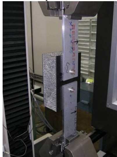
Figure 3. Insert shear test.
