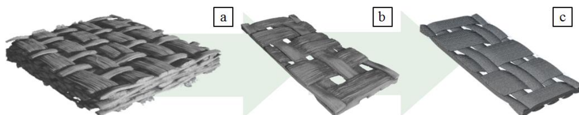
Figure 6. Rendered micro CT-scan images of the full laminate slice (a), the RVE (b) and the corresponding finite element RVE of the fabric (c)
