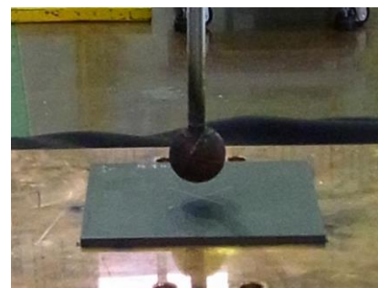
b) Discharge probe with insulating sphere
