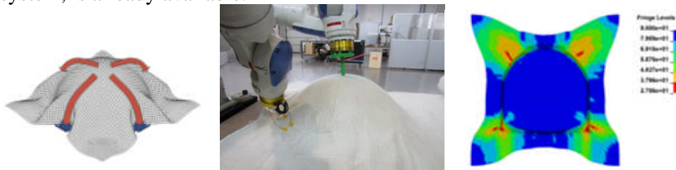
Figure 6. Simulated robot draping strategy and preliminary robot draping test with robotic grippers
