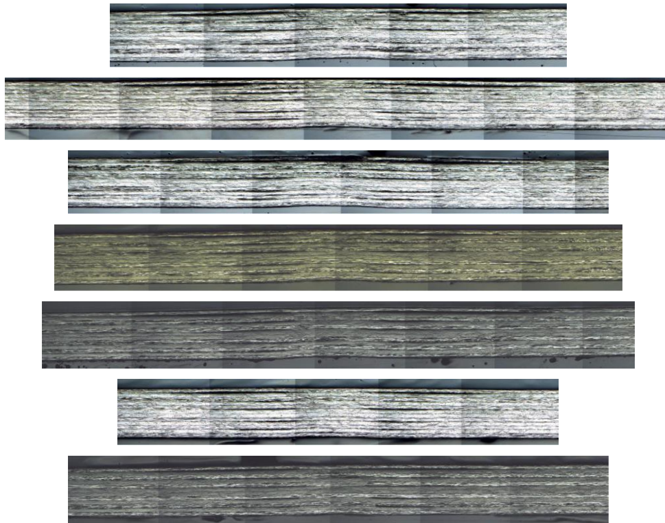
Figure 2. Optical microscope photographs of specimens A1, B5, C1, D1, E1, F3, G5 (from top to bottom) sectioned along the 0° direction through the impact point. The impacted face of laminates is on the low side of each picture.
