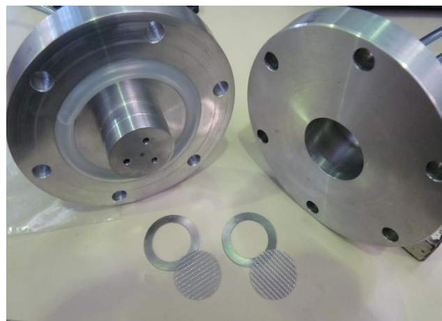
Figure 3. Test bench for out of plane permeability measurement.
