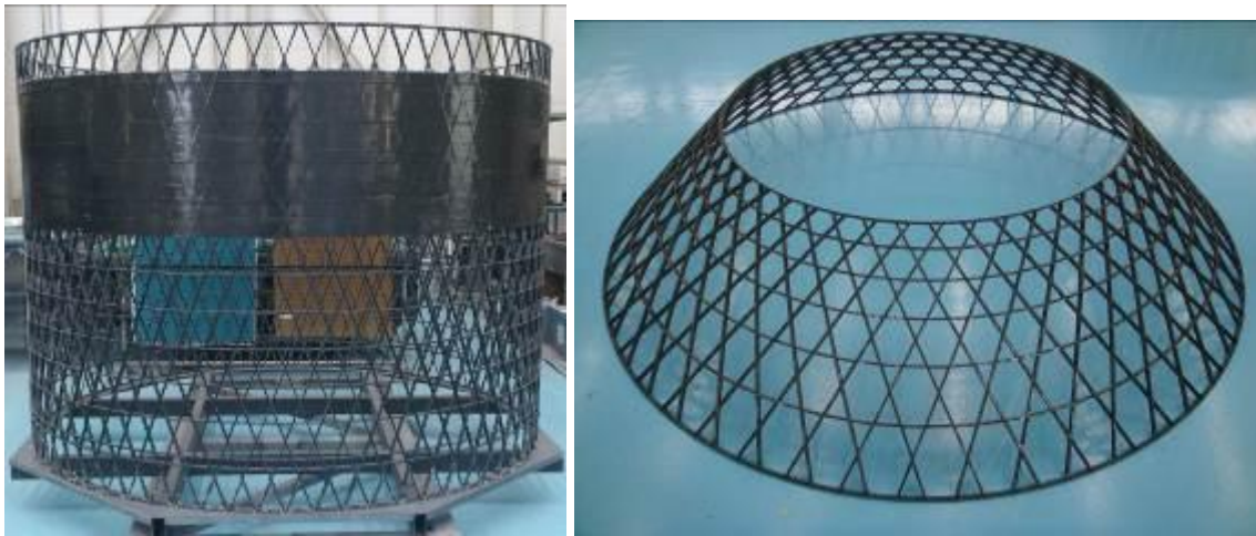
Figure 8. The manufacturing results of demonstrators. (Left : Cylindrical with skin, Right : Conical)
