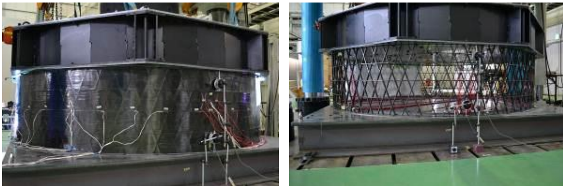
Figure 11. The test setups for cylindrical demonstrators with and without skin.
