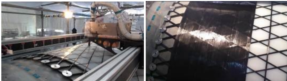
Figure 6. The winding process for cylindrical demonstrator and its skin.
