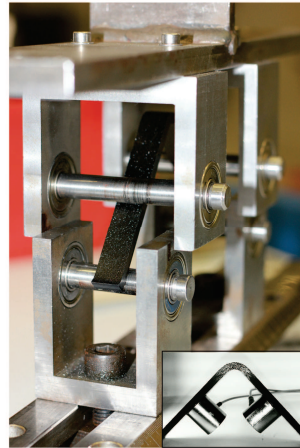
Figure 1. Rig used for the static and fatigue testing. Inset: the acoustic emissions sensors attached to the specimen.
