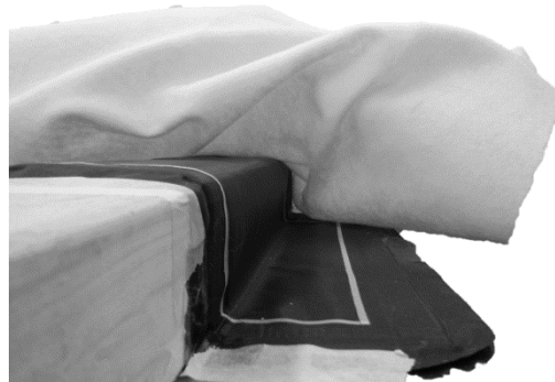
Figure 1. Flexible sensor and breather fabric laid up on C-section tool.
