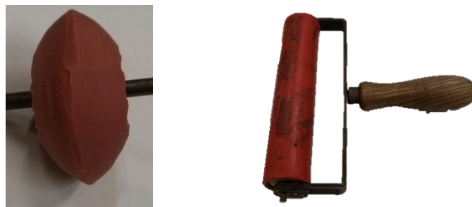
Figure 4. Left , compliant silicone roller. Right , conventional roller.
