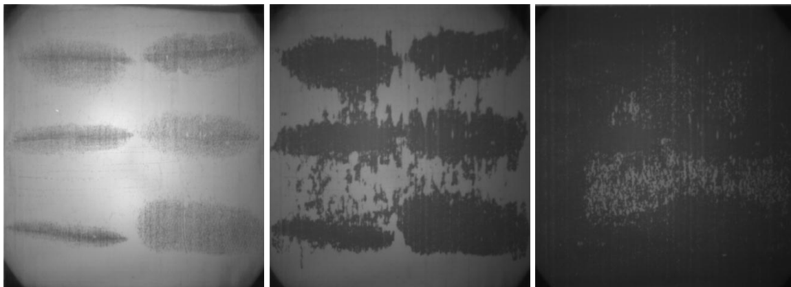
Figure 7. Left, Ply as laid down using 6 different conformable rollers. Centre, ply after 1 hour relaxation in cleanroom conditions. Right, ply after 20 minute debulk, with trapped air pockets visible between roller passes.
