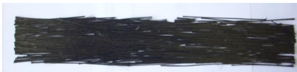
Figure 1a. Realigned carbon fibre stripes
