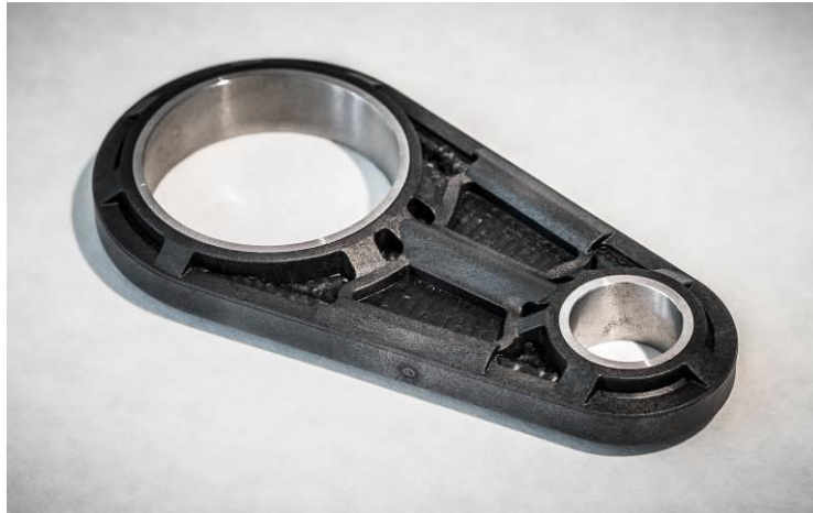
Figure 1. The torque arm, made of glass fibre/PA 6.6 which is used as a demonstrator. The black colour is caused by the additional material applied by the final injection moulding step.
