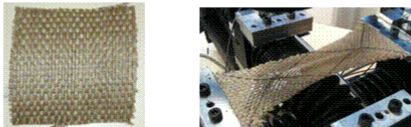
Figure 1. Flax woven (a). Bias-test (b)
