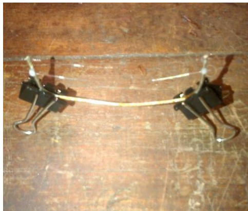
Figure 1. Single glass fibres with PA6 fibre tied and mounted on metal frame
