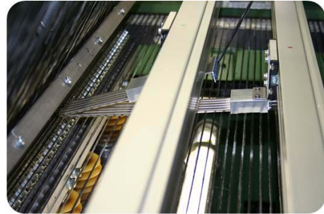
Figure 02. Side view warp yarn shogging device for selective manipulation of the warp yarn course
