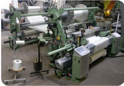
Figure 05. P1 weaving machine with open reed (ORW) and warp yarn shogging device
