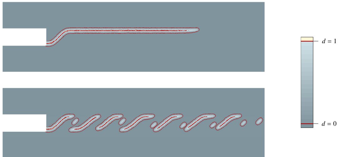
Figure 7. Damage profiles from thick level set method with Y_c as only parameter (top) and with additional parameter Y_0 (bottom).
