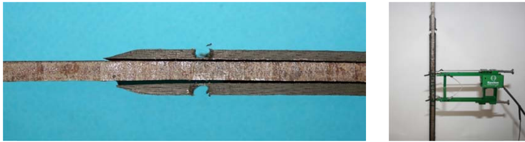
Figure 3. Cut off CFRP strap edge (left) and typical S-100 specimen during testing (right).
