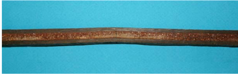
Figure 8. Misalignment of A-100 specimens.
