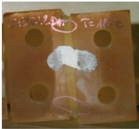
Figure 3. Shear test done at 125°C. The white spot was used for video-control of strain evolution. Plasticity is obtained after cooling.
