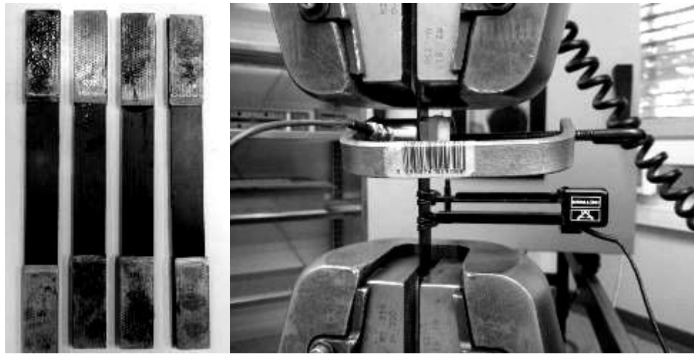
Figure 4. Specimens for laminates [0_2/30_2]_S and the experimental installation with AE sensor
