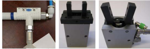
Figure 1. A vacuum cup with an ejector system (left). Two examples of clamping grippers (right).
