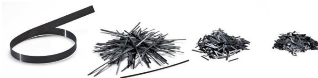
Figure 2 From left to right: unidirectional tape, chips with length 150 mm, 30 mm and 10 mm.
