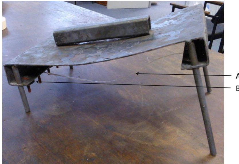
Figure 2 5 Bundles Steel Rig. A) GF Bundle. B) Nut, bolt and washer.
