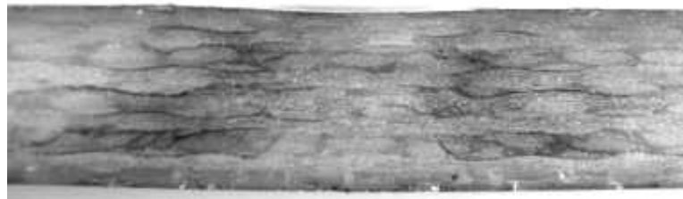
Figure 11. Transversal section of impact area. Delaminating cracks highlighted by black ink.
