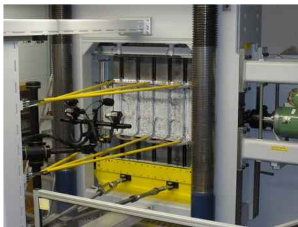
Figure 5. Test rig with frame stiffened panel, frames supported by guiding rods, ARAMIS-DIC in front and rear (not visible)
