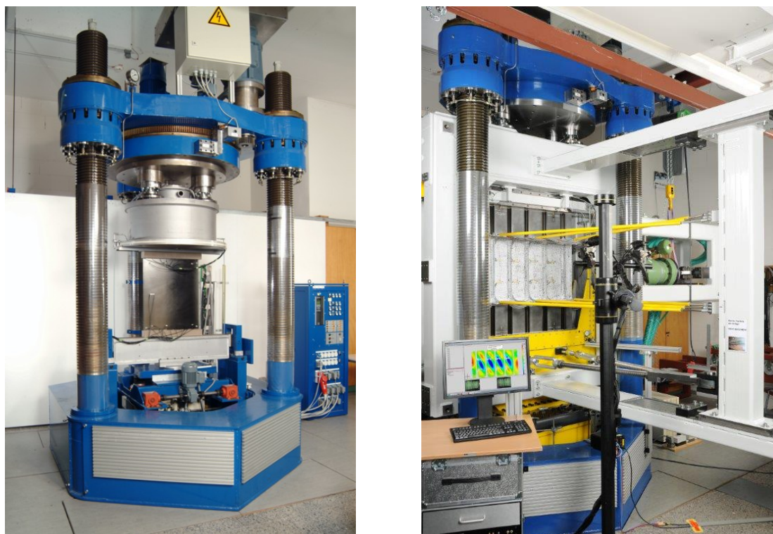
Figure 1. Buckling test facility: axial compression configuration (left); extended facility in shear compression test rig configuration (right)
