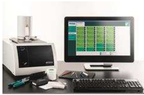
Figure 1: Work station with a DSC 214 Polyma with automatic sample changer, PC with touch screen for pre-defined methods and several tools for sample preparation
