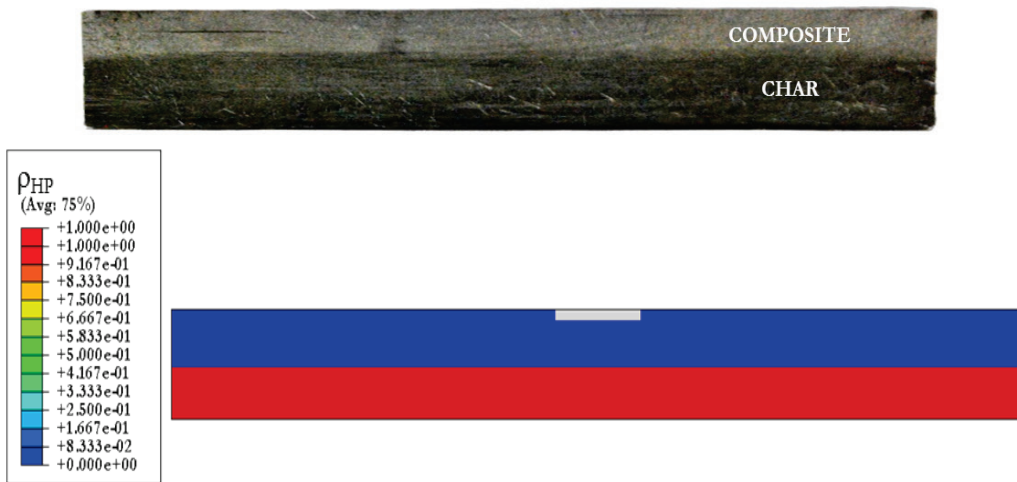
Figure 6: Micrography of the composite sample subjected to fire (top), initial conditions for simulation: uniform damage field (bottom, red = full damage, blue = undamaged material)
