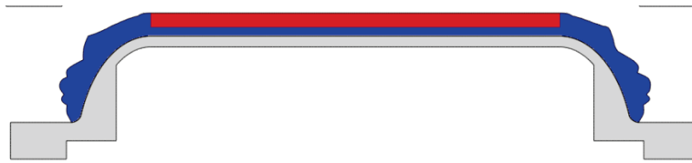
Figure 8: tank geometry (red = fully damaged composite, blue = undamaged composite, grey = liner + metallic bosses)
