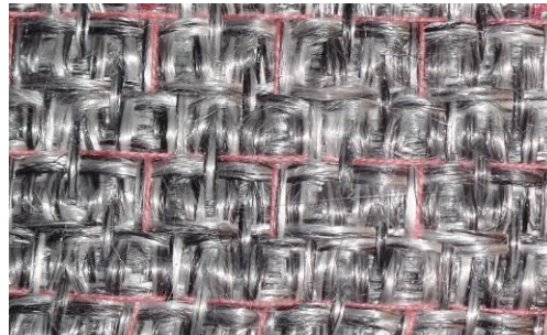
Figure 4. Detailed view of a woven preform with tracers
