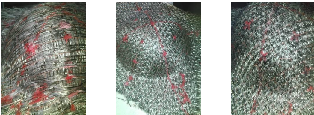
Figure 2. 3D warp interlock formed fabrics with different architectures as: a - Through the Thickness, - b - Layer to Layer, c - Orthogonal
