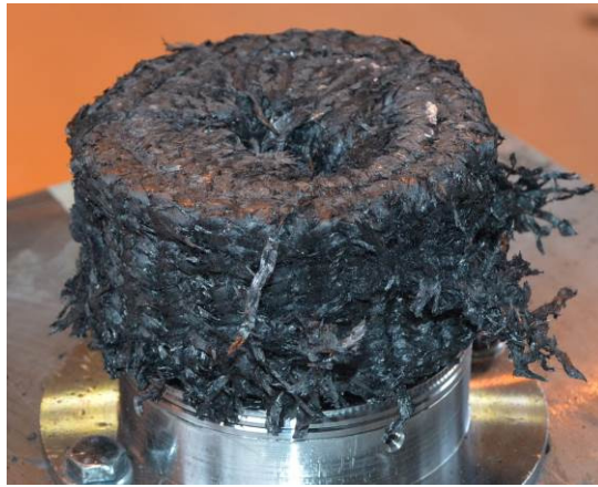
Figure 3. Carbon/PA6 conical crashbox after test
