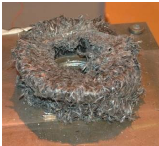
Figure 4. Glass/PP cylindrical crashbox with 75° bias fibers after test
