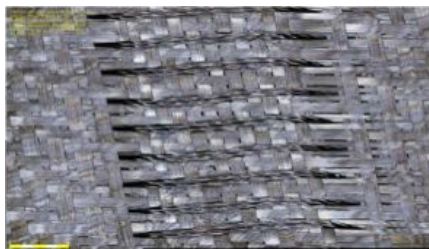
Figure 7. Severe fiber misalignment on bottom side of a dry preform
