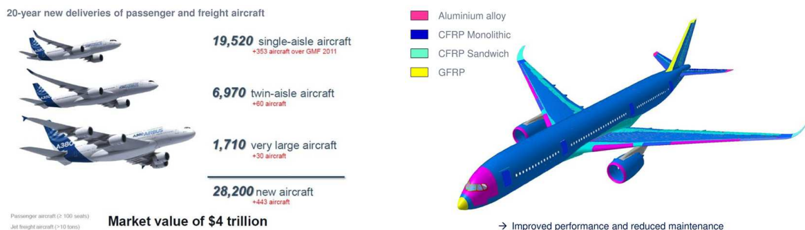
Figure 1. Left: 20-year demand for 28.200 new passenger and freight aircraft [2], Right: A350 XWB composite applications [3]
