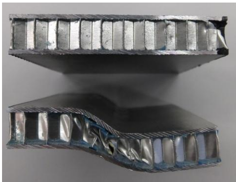
Figure 2. Undamaged AHS ( d=6 mm) panel and another one after edgewise compression test.
